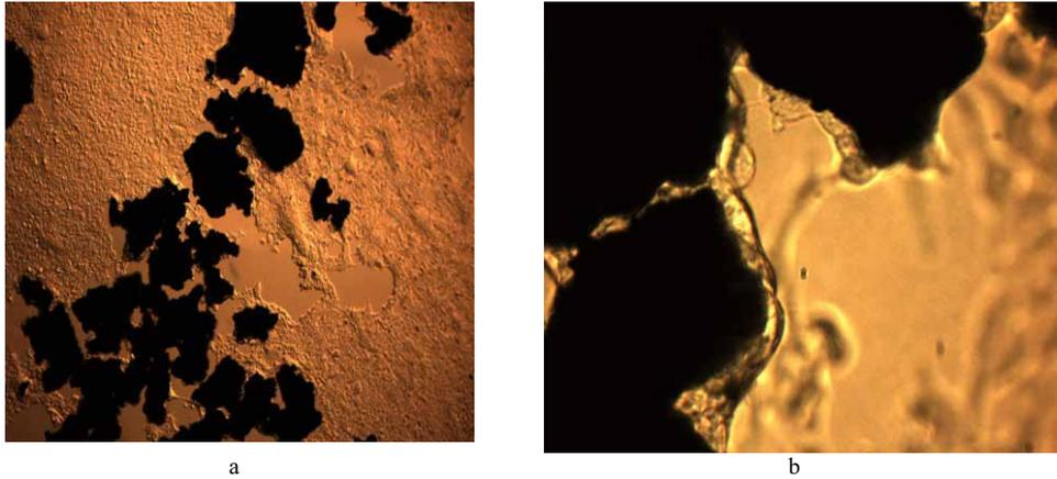
**Fig. 3** The biological tests on bio-adaptability of the powdered NiTi *in vitro*. The photos show that the culture of living human liver cells not only survive in contact with NiTi (a), but tend to change the place from standard biocompatible substrate to particles surface (b).
