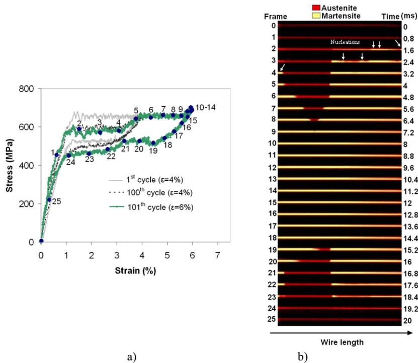
Fig. 5. NiTi wire phase transformation fronts evolution during complete SIM transformation previously cycles 100 times up to half of the transformation. Strain rate  $10 \text{ s}^{-1}$ . a) Stress-strain curve. b) Thermographic pictures taken every 0.8 ms.
