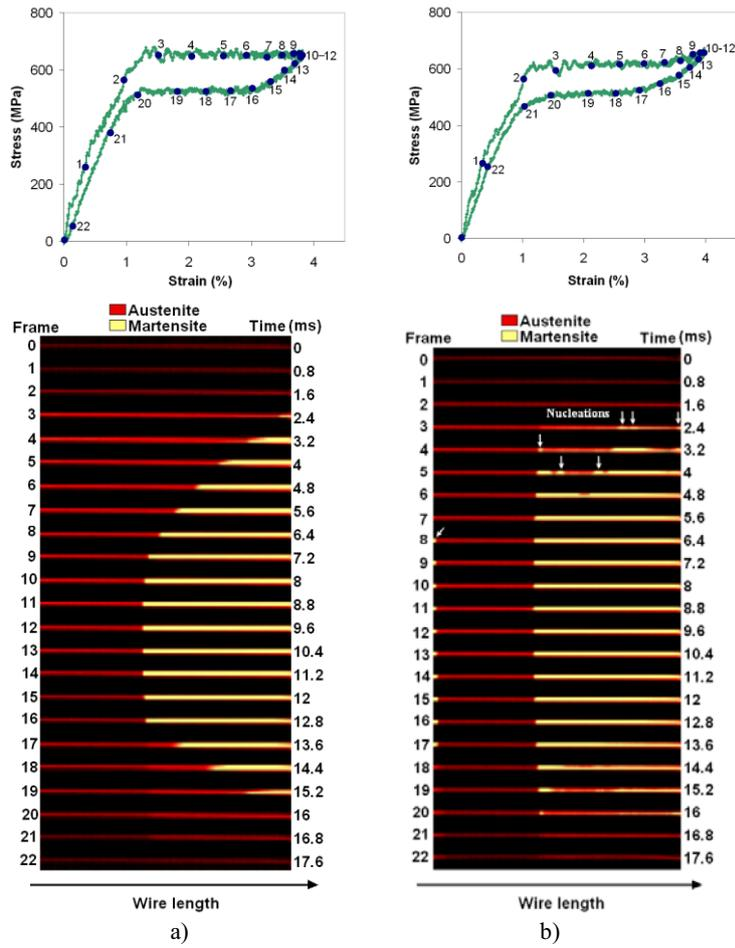
Fig. 4. NiTi wire phase transformation fronts evolution during the deformation up to half of the SIM transformation at impact strain rate ( $10 \text{ s}^{-1}$ ). a) 1<sup>st</sup> cycle. b) 50<sup>th</sup> cycle.
