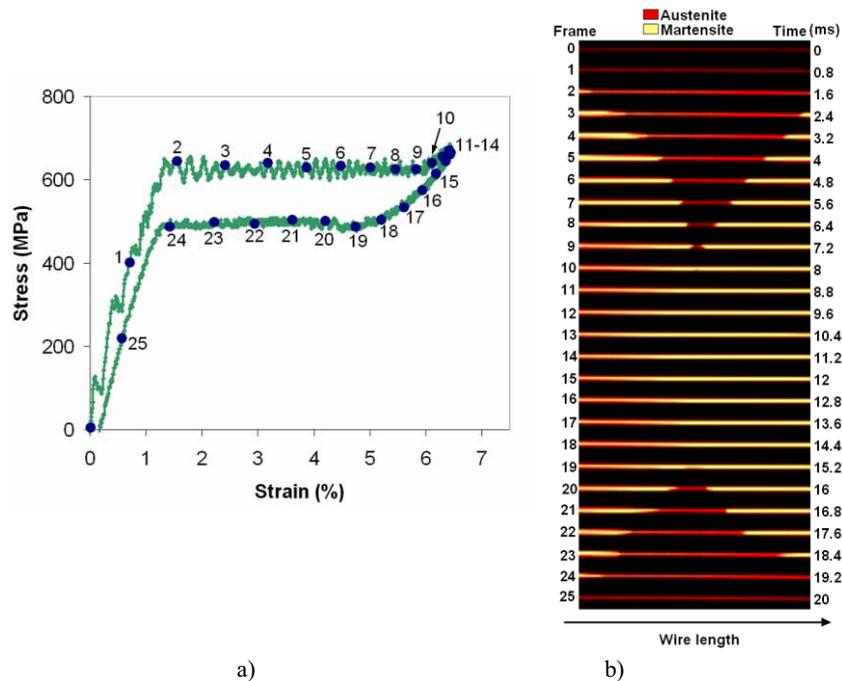
Fig. 2. NiTi wire phase transformation fronts evolution during the complete martensitic transformation ( $\epsilon=6.5\%$ ), induced at impact strain rate ( $10 \text{ s}^{-1}$ ). a) Stress-strain curve. b) Thermographic pictures taken every 0.8 ms.
