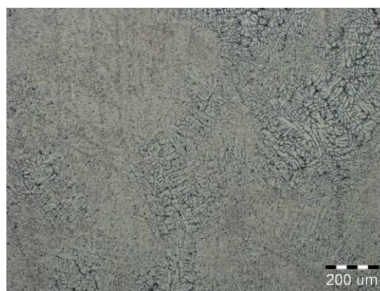
Fig. 4. Alloy B, induction melting, 100x, OM
