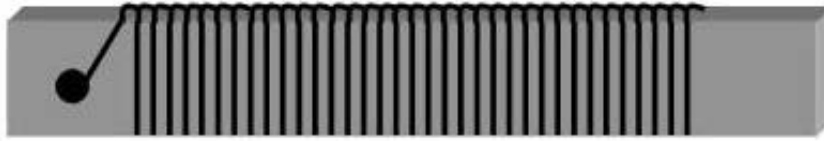
Fig. 1 A scheme of a fixture for shape-setting of the SMA hooks.
